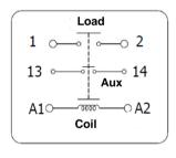
Note: The coil, load and Aux. have no polarity
