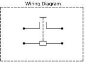
Note: No polarity on the load and coil
