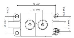
Remark: in case of no tolerance shown in outline dimension: outline dimension  $\le 10$ mm; tolerance should be $\pm 0.3$ mm, outline dimension > 10mm and  $\le 50$ mm, tolerance should be $\pm 0.5$ mm, outline dimension > 50mm, tolerance should be $\pm 0.8$ mm.
