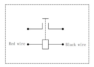
Note: No polarity on the load and coil
