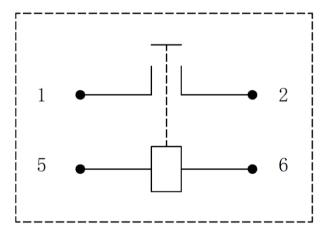
Note: No polarity on the load and coil
