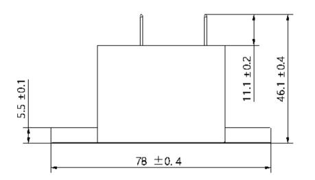
Coil input terminal(Non-polarity) #250insert terminal,Thickness=0.8 Load input terminal(Non-polarity) #250 insert terminal,Thickness=0.8
